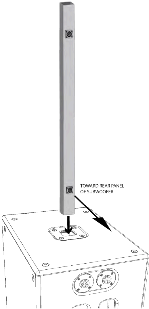
Figure 83. Installing the 95 cm Active Speaker Tube on the SUB310.
