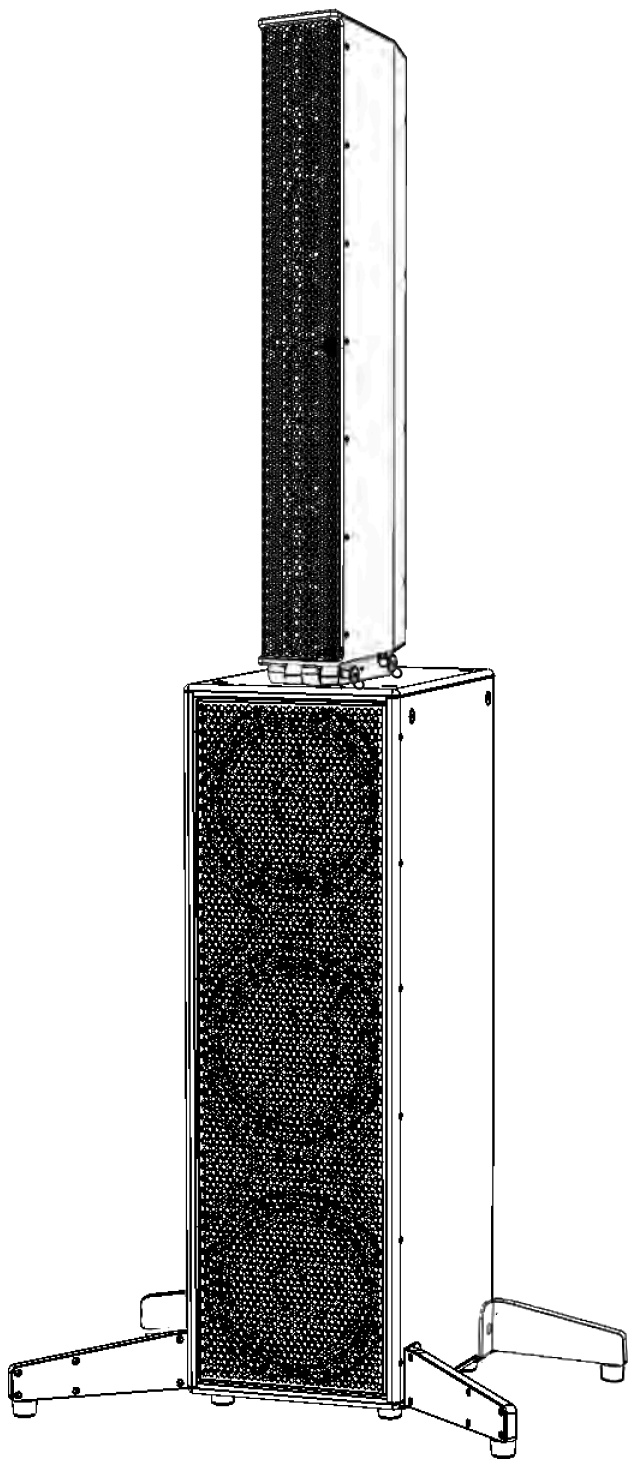
Figure 135. LCC84 deployed atop SUB310 using the Tower Rigging System.
