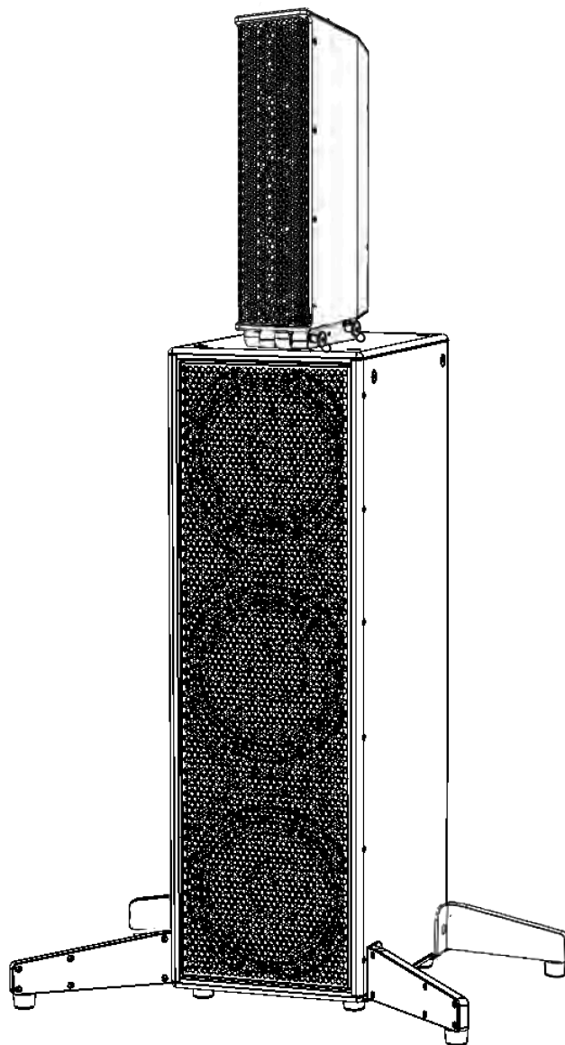
Figure 136. LCC44 deployed atop SUB310 using the Tower Rigging System.
